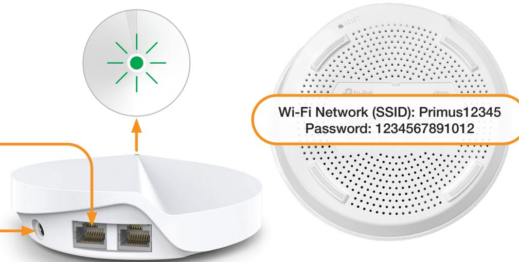
⚠ If the light is **red**, reboot the modem and Wi-Fi pod by unplugging the power adaptors.
